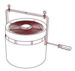
The Onyx Series system is designed to hang vertically and freely 12-to-18 inches, or as close as possible, from the ceiling on professionally installed hardware, for models 10/15/25, capable of supporting a minimum of five times the weight of the Onyx Series unit, 60 lb. (27 kg.). Example - 1/4" (7 mm) diameter steel bolt is rated at 60 lb. (27 kg.) load.
