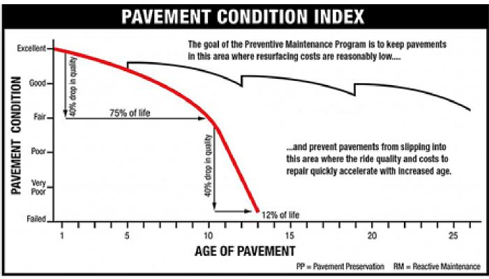
To Use simplistic terms, with a PCI of 62 our average road has used up 75% of its useful life. To be sustainable, it needs to be 50%. Roads deteriorate very quickly when they are allowed to get a PCI less than  $\sim$ 55
