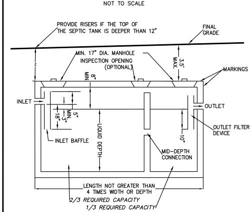
CONCRETE SEPTIC TANKS SHALL CONFORM TO SECTION V. "SEPTIC TANKS" OF THE "CONNECTICUT PUBLIC HEALTH CODE, REGULATIONS AND TECHNICAL STANDARDS FOR SUBSURFACE SEWAGE DISPOSAL SYSTEMS", REVISED THROUGH JANUARY 1, 2018
